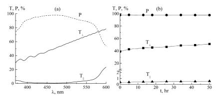
Figure 10: (a) Polarized transmittance  $(T_{\perp}, T_{\parallel})$  spectra and the degree of polarization (P) of 8.8- $\mu$ m-thick polarizing film obtained by stretching and subsequent annealing of PVA–TPA nanocomposite film, (b) the optical properties of this film at  $\lambda=466$  nm as a function of its residence time in hot humid air  $(60^{\circ}\text{C}, 90\% \text{ RH})$ .
