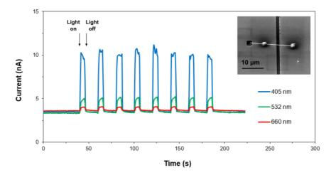
Figure 9: Measured photoresponse of CdS nanowire photodetector for different wavelengths ( $I = 3 \text{ W/cm}^2$ ). Inset: Scanning electron microscope image of the photoresistor.
