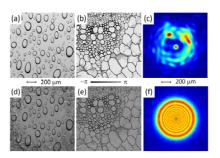
Figure 13: Simulation results of ws-PIE(a) Original modulus and (b) phase transmission image of the object. (c) Simulated diffraction pattern with 700 nm illumination. (d) and (e) are modulus and phase images reconstructed using ws-PIE obtained from 10 diffraction patterns at 10 nm scanning step beginning at 700 nm. (f) Represents the recovered illumination amplitude in the object plane for 750 nm.
