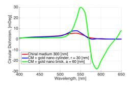
Figure 15: Circular dichroism spectra for chiral layer of HgS nanocrystals (h = 300nm and period = 110nm) and enhancement of circular dichroism of HgS nanocrystals inside the periodic array of golden nanocylinders (r = 30nm) and nanobricks (a = 60nm).
