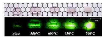
Figure 4: Upconversion luminescence in oxyfluoride glass and glass ceramics samples under excitation at 980 nm.
