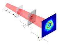
Figure 12: Schematic of the setup for ws-PIE. Diffraction patterns were recorded by repeating the exposure with different wavelengths. The distance between the pinhole and sample is z1. The diffraction patterns are collected by a two-dimensional detector placed at z2 away from the sample.
