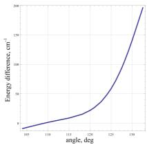
Figure 19: Energy difference between the ground and first exited states of UO<sub>3</sub> molecule.
