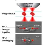
Figure 17: Aggregation force measurement between two trapped RBCs.
