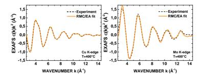
Figure 5: Example of RMC/EA calculations for the Cu and Mo K-edges EXAFS spectra of  $\alpha$ -CuMoO<sub>4</sub> at 400°C. Dashed lines - experiment, solid lines - fit.
